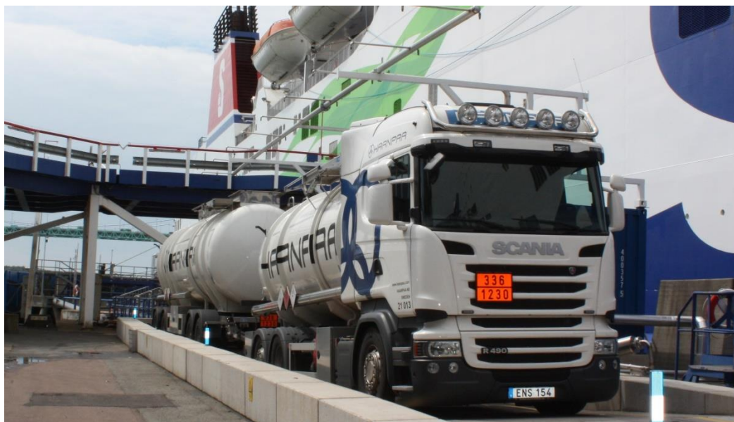
Figure 12: Stena Germanica bunkering methanol from a tanker truck with trailer (photo: J.Ellis)
