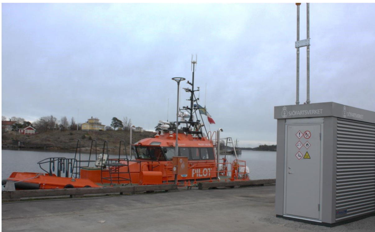
Figure 14. Swedish Maritime Administration methanol-fuelled pilot boat with methanol M97 dispensing station shown on the right (see Figure 18 for complete view of methanol M97 bunkering station)(Photo: J.Ellis).
