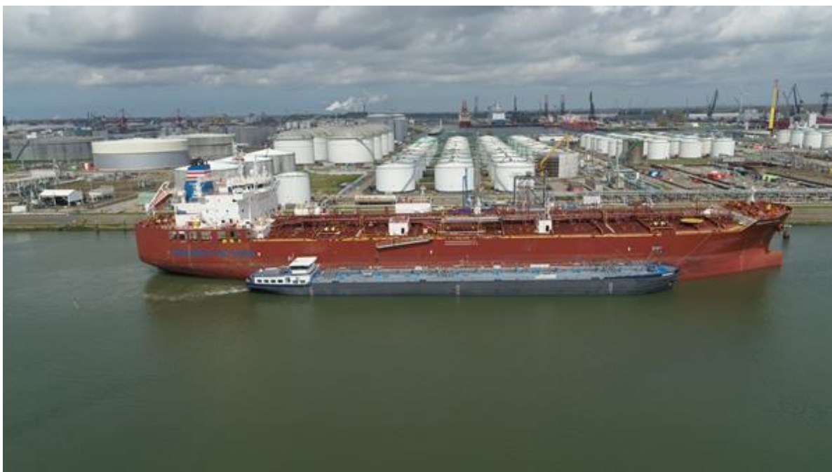
Figure 13: Methanol barge to ship bunkering in Rotterdam at the VOPAK Botlek terminal (photo courtesy Methanex).
